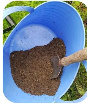
Fig. 2. Mix all samples from a single site together.
